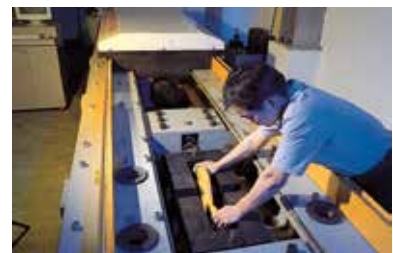
Tensile Test, Capacity 300 tonnes
