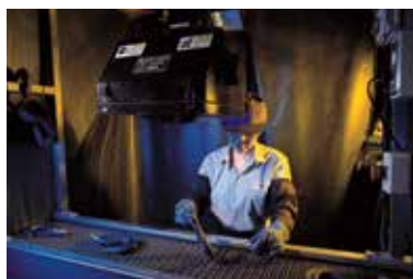
Magnaflux Crack Detection
