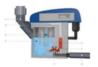
MAC180-T dryer and largers are equipped with a zero loss drain system, interfaced to the DMC24, to assure the drainage of the condensed water only with no air loss.
